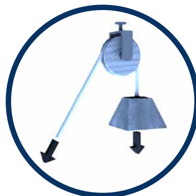
This pulley system changes the direction of a force. To lift the weight up, you must pull down.
