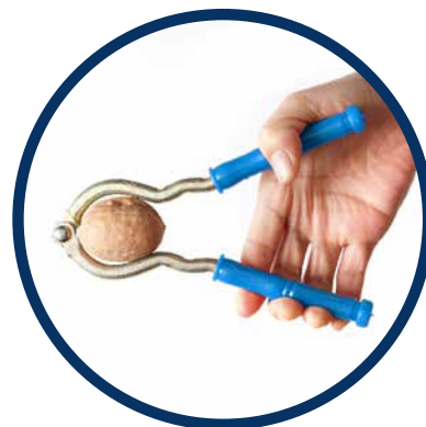
A nutcracker reduces the amount of effort (input force) required on a load (the nut).
