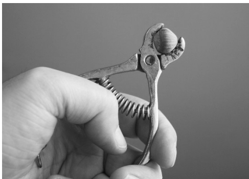
A nutcracker reduces the amount of effort (input force) required on a load (the nut).
